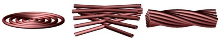
Figure 1 Geometry of the DTI phantoms used in this study: Rings, kissing fibers, twisting fibers
